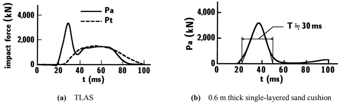
Figure 2 Comparison of impact forces obtained using two absorbing systems
