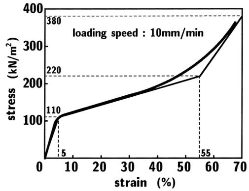
Figure 5 Stress-strain relation of EPS layer
