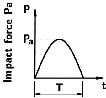
Figure 4 Assumed impact force wave onto RC core slab
